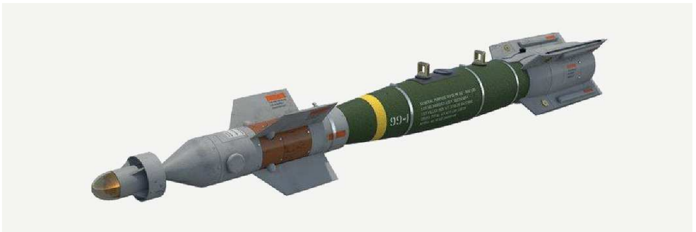
Mk.82 500 lbs bomb equipped with laser kit.
