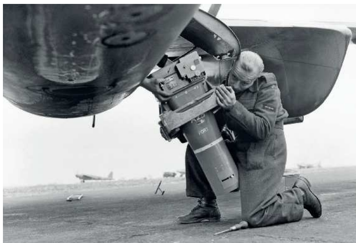
Installation of an F52 camera and 36" Lens in a PR Mosquito. (IWM)
