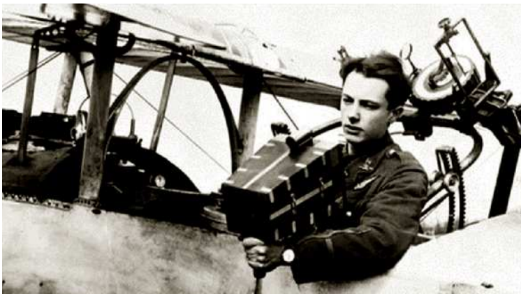
RFC BE.2.C with side-mounted camera (1916).
