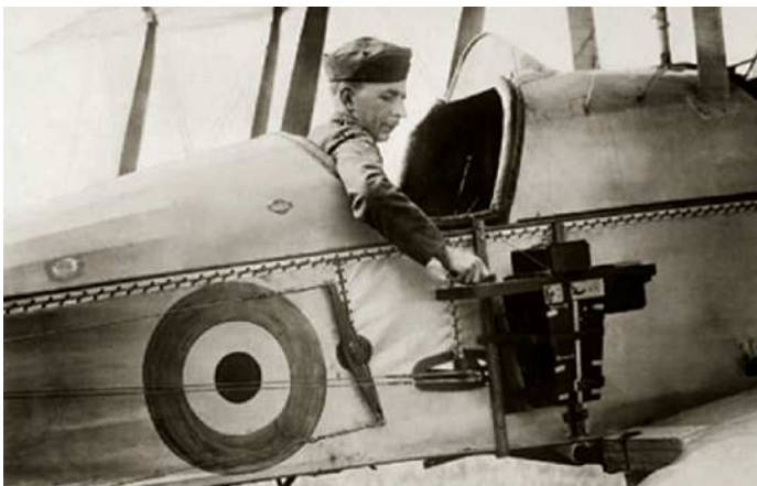
RFC BE.2.C with side-mounted camera (1916).
