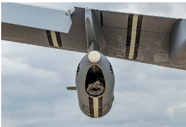
Wing pod on the A330 MRTT, housing the hose and drogue system.
