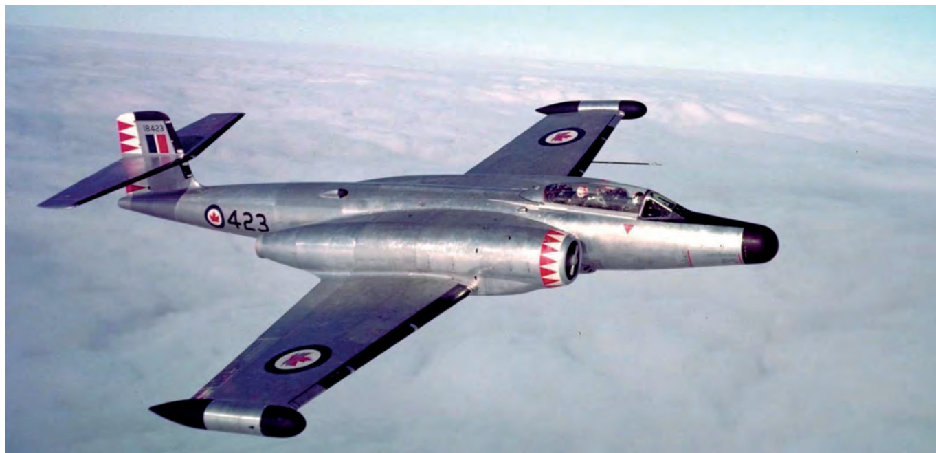
CF-100 equipped with wingtip rocket pods.
