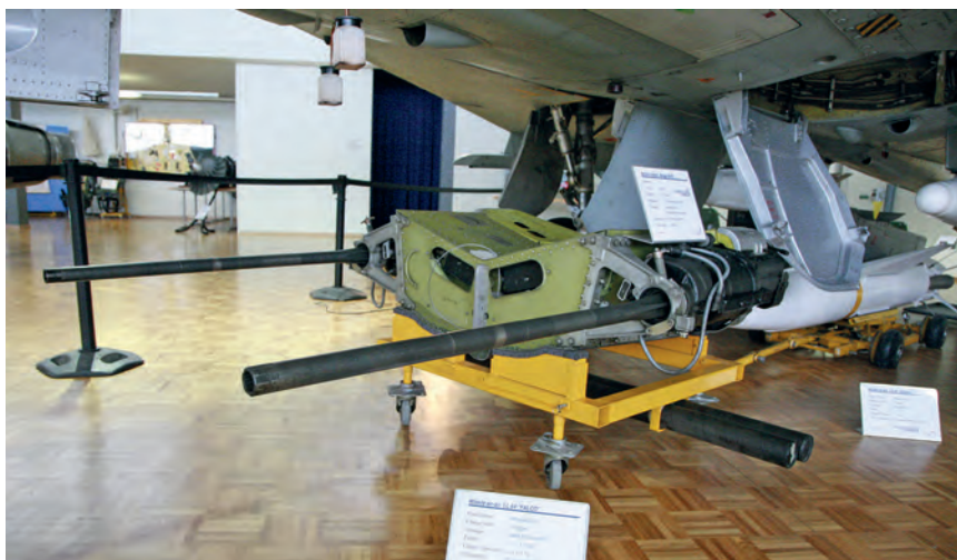
The Belgian A.F. Mirage 5 was equipped with the DEFA 30 mm gun pack.
