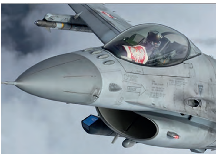
The mouth of the 20 mm Vulcan just above the left hand wing strake.
