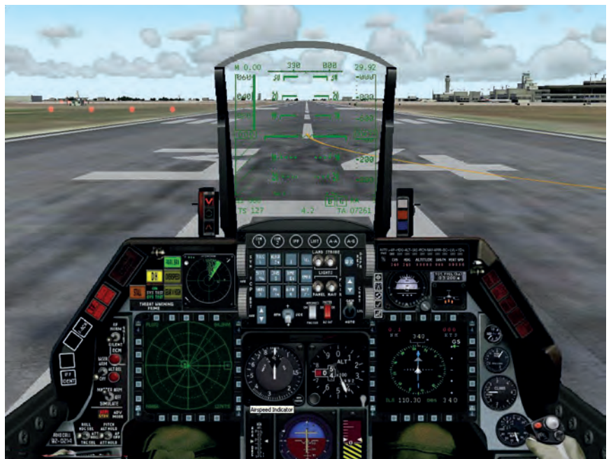
F-16 cockpit with two MFD (Multi Function Display) and HUD (Head-Up Display).
