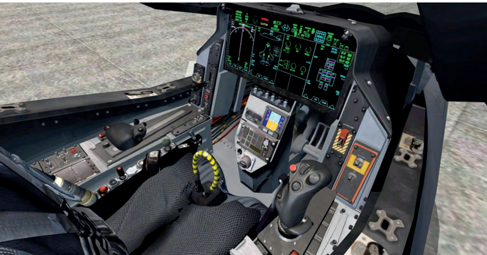
The F-35 glass cockpit with multifunctional touchscreen.
