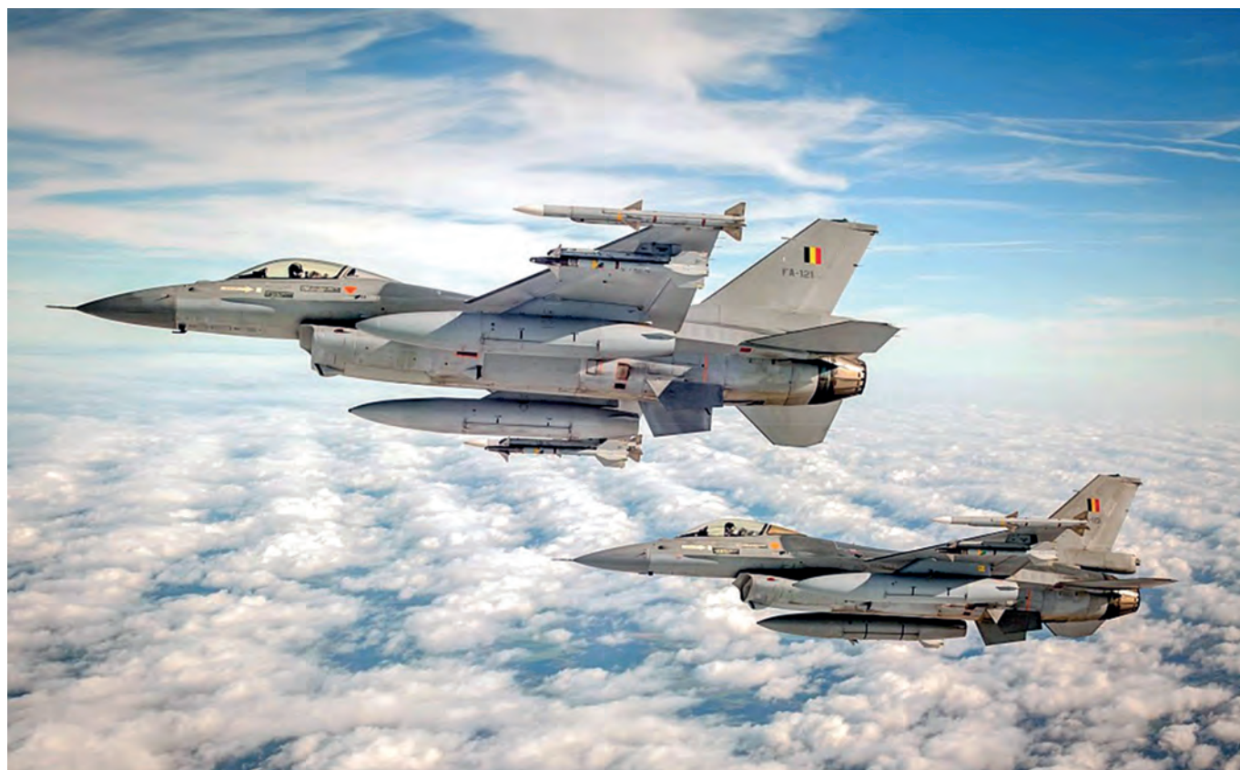
Belgian F-16's with each two AIM-9 under the wings and AIM-120 AMRAAM on the wing tips.
