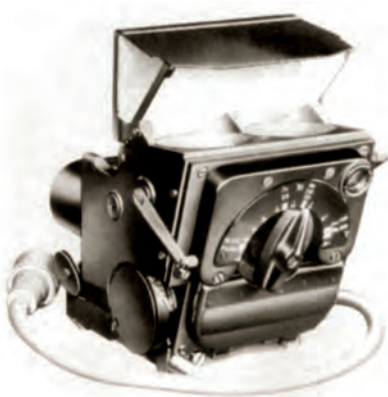
Ferranti Gyro Sight Mk.IIc. Already in use in several WW2 fighters.
