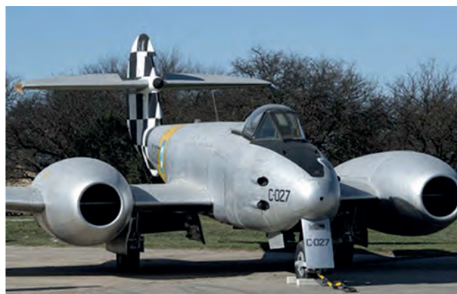
Gloster Meteor F4, four 20 mm HS cannons in the nose.
