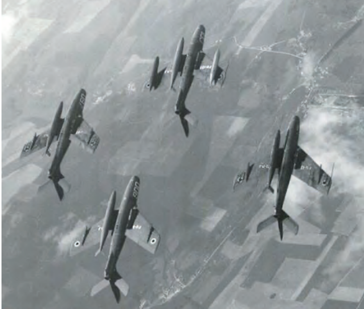
Aerobatic exercises in the proximity of Florennes. Photographs taken in 1966 by Jean-Pierre Quodbach (42 Sqn Bierset). Note the asymmetrical fuel tanks. The opposite pylon is kept free for attaching a special weapon.
