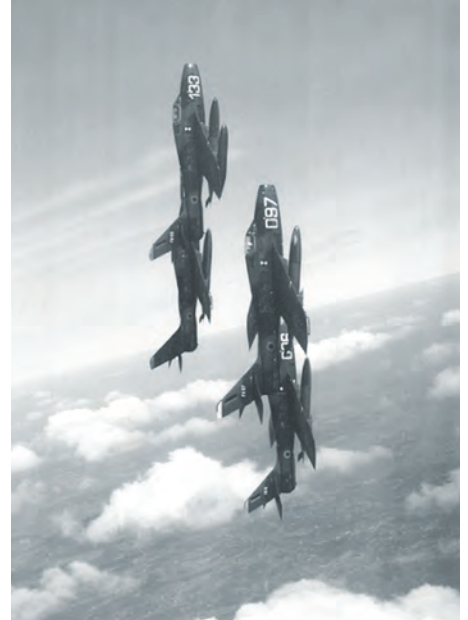
Aerobatic exercises in the proximity of Florennes. Photographs taken in 1966 by Jean-Pierre Quodbach (42 Sqn Bierset). Note the asymmetrical fuel tanks. The opposite pylon is kept free for attaching a special weapon.
