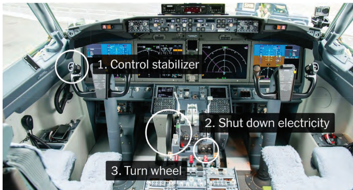
B 737 MAX MCAS Cut-off switches.
