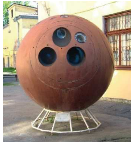
Re-entry capsule, showing camera ports.
